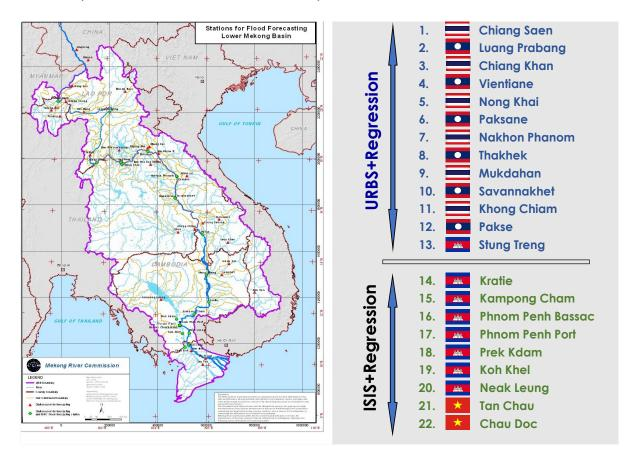
Figure 6: Key stations and model application for River Monitoring and Flood Forecasting.
